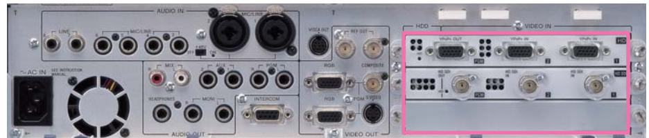
Rear Panel Connectors of AWS-G500HD
