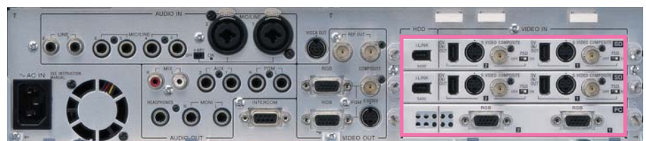
Rear Panel Connectors of AWS-G500HD
