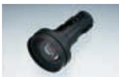
VPLL-ZM31 ■ 1.1 times zoom short focus lens ■ Throw ratio: 1.55-1.62:1
